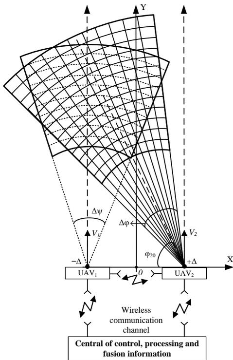
Fig. 2. Front-area mapping with a two-position small OBRs
