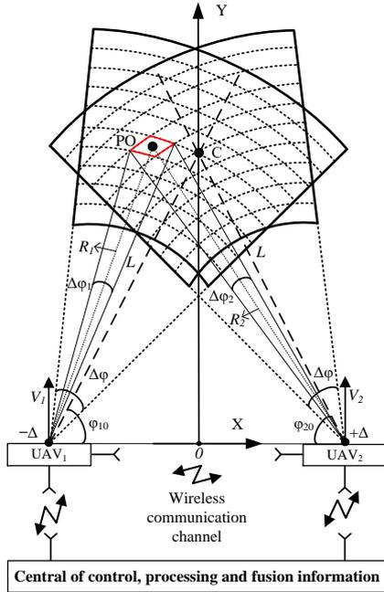
Fig. 1. Resolution elements of a two-position small OBRs
