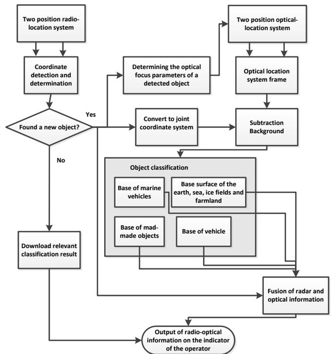
Fig. 4. The block diagram of the algorithm for information fusion
