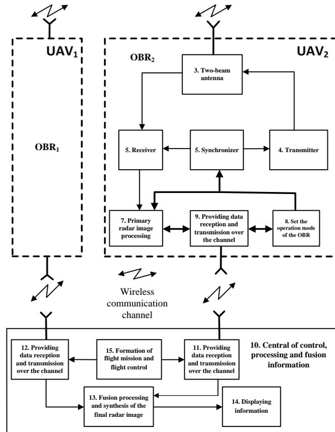
Fig. 3. Function diagram of two-position system small OBRs for mapping of laying surfaces in the front-side area
